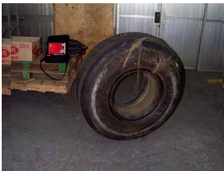
Fig. 1-13 White Marks on Left Sidewall
