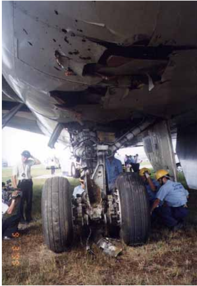
Fig. 1-1 Damage to Fuselage
