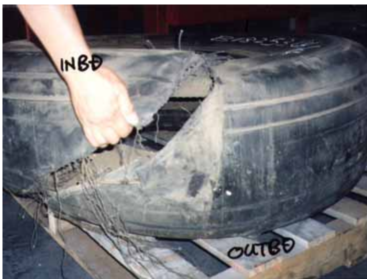
Fig. 1-12 Left Tire Damage and Tread Abrasion
