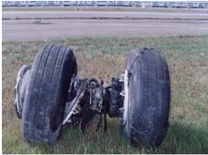
Fig. 1-3 Damage to Front Truck of Left Body Gear
