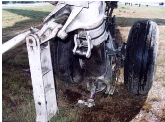
Fig. 1-4 Damage to Rear Truck of Left Body Gear
