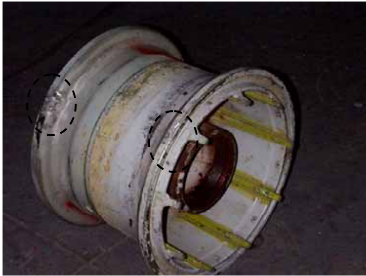
Fig. 1-8 Spot-like Abrasion Marks (circled areas)
