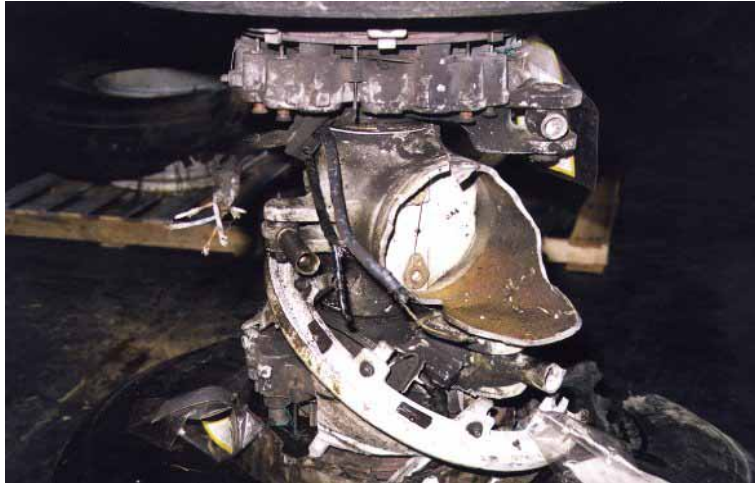
Fig. 1-22 Damage to Front Body Gear Truck
