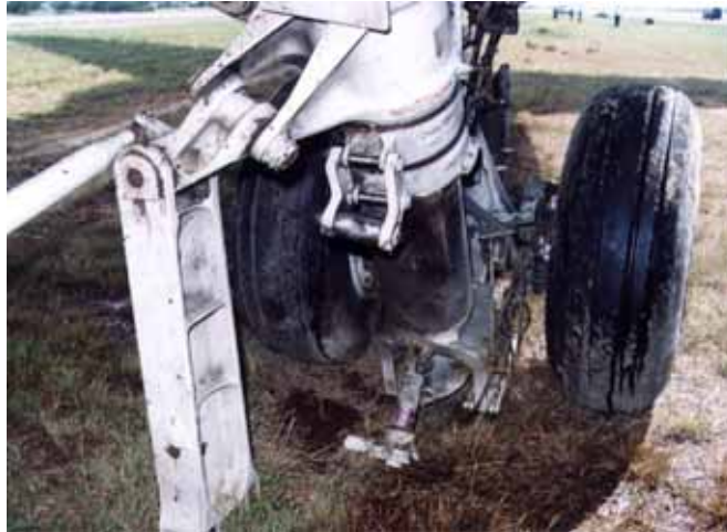
Fig. 1-24 Damage to Rear Body Gear Truck
