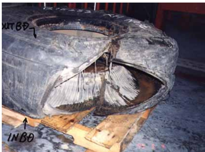
Fig. 1-18 Damaged Right Tire and Tread Abrasion
