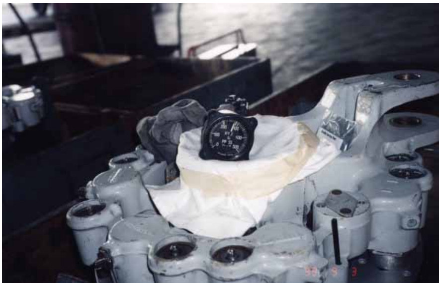
Fig. 1-28 External Pressure Gauge Indicated 3000PSI
