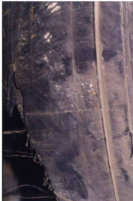
Fig. 1-20 Abrasion Vertical to Grooves
