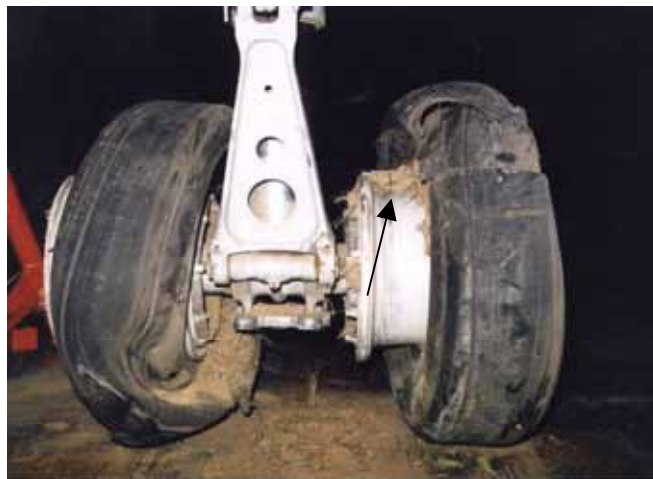
Fig. 1-11 Left Wheel Hub Covered with Mud (pointed area)
