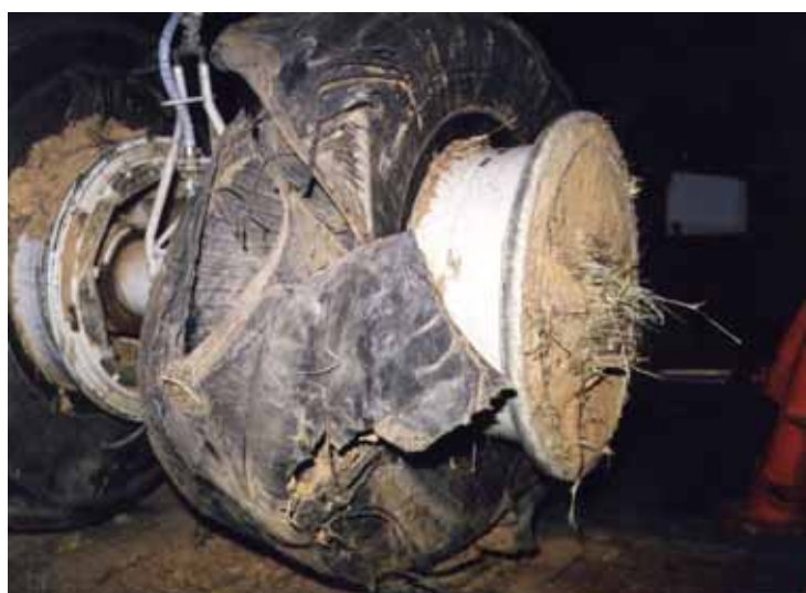
Fig. 1-17 Hub's Right Side Covered with Mud
