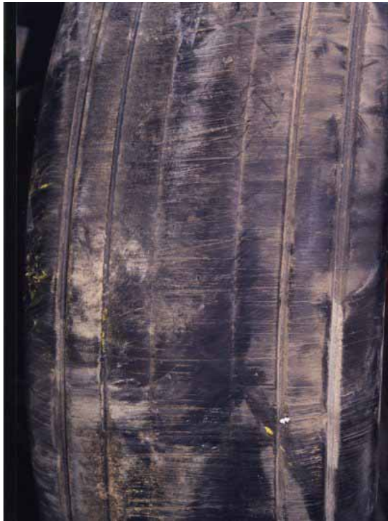
Fig. 1-14 Tread Covered with Abrasion Vertical to Grooves
