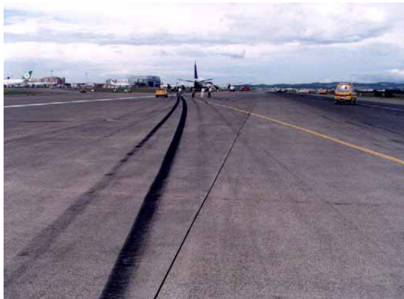
Fig. 1-34 Ground track between 150-180 meters.
