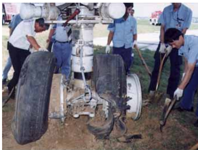
Fig. 1-2 Damage to Nose Wheels
