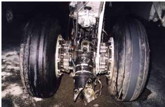
Fig. 1-23 Rear Truck Snapped at 45° Angle
