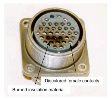
Metallurgical examination of the burned pin-clamp couplings indicates that they were manufactured correctly and that there was no presence of contamination on the contact surfaces.
