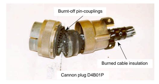
The investigation also showed that several of the contact pins were discolored due to the overheating and that the insulating material between the pins in the cannon plug had been affected by high temperature and had also been discolored. This all points to the fact that the source of heat generation was not external in connection with the fire but took place within the electrical pin couplings during an extended period of time.
