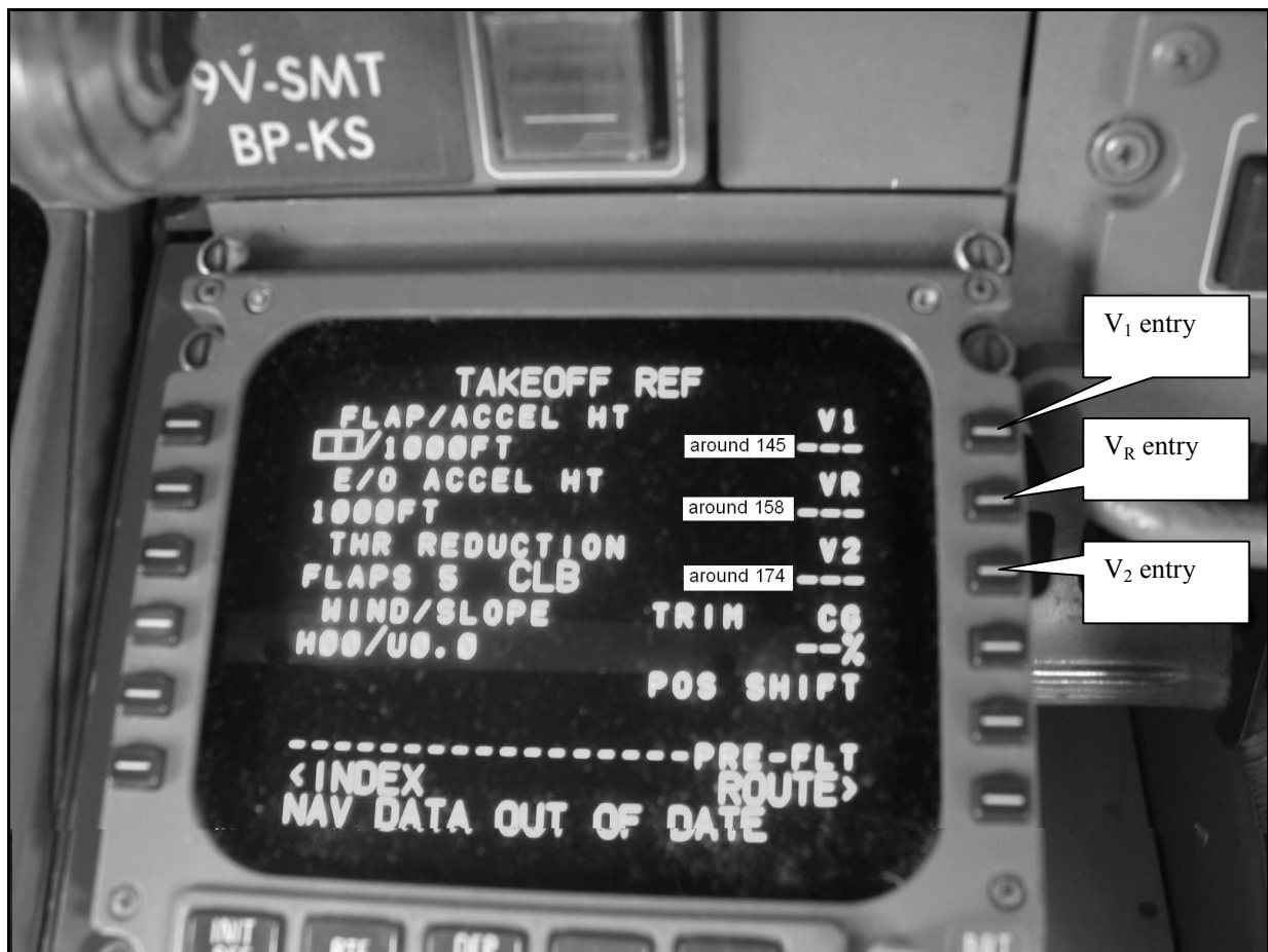
Figure 3 9V-SMT FMC display of V speeds
