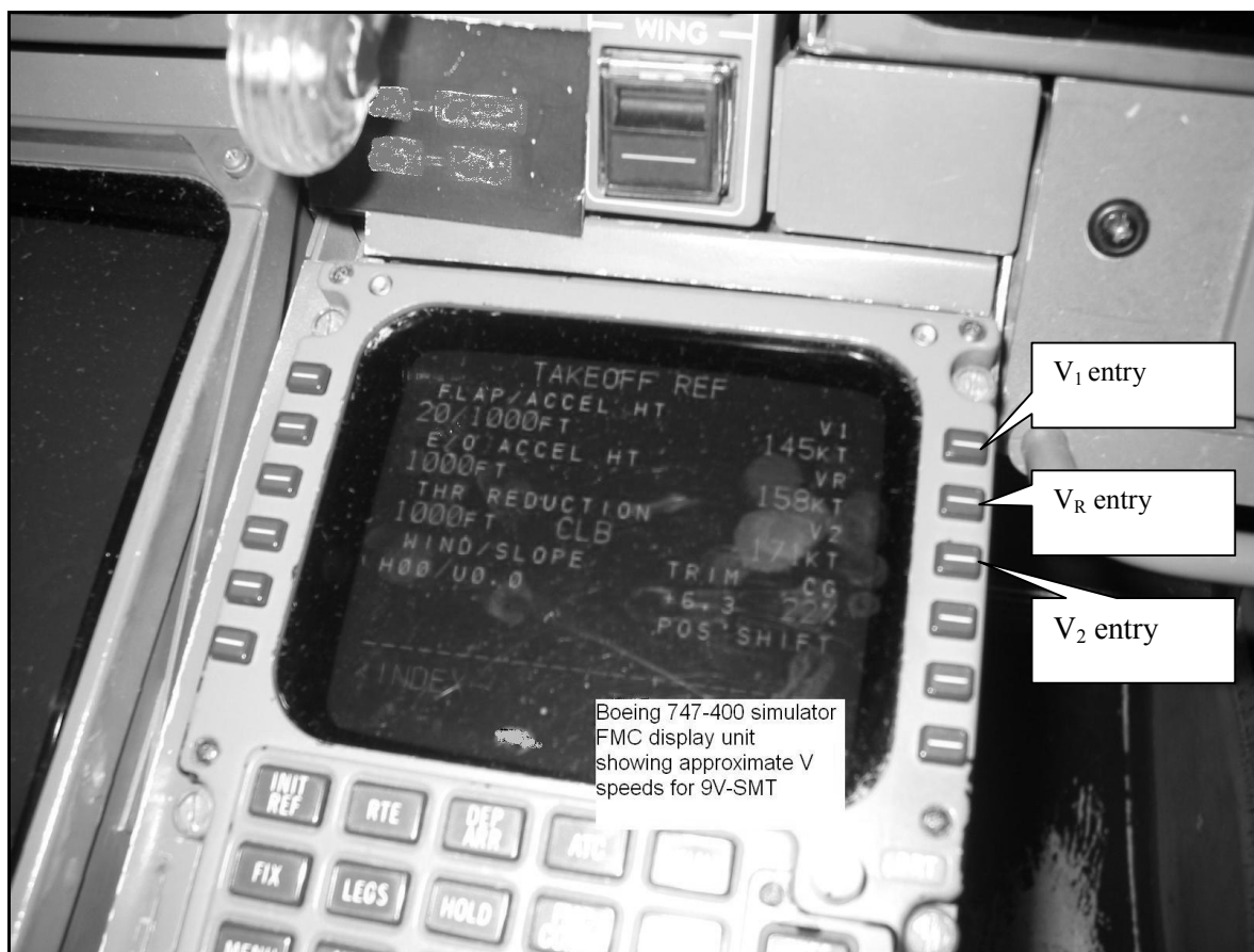
Figure 5 Boeing 747-400 simulator FMC display
