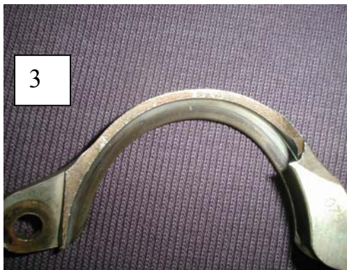
Photo 1: The 14 th Stage Manifold on a tool rig Photo 2: The failed manifold coupling position Photo 3: The fractured clamp
