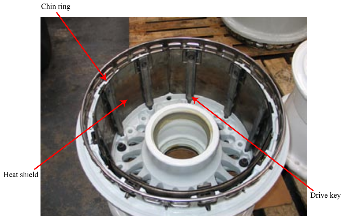
Figure 4 Construction of main wheel
