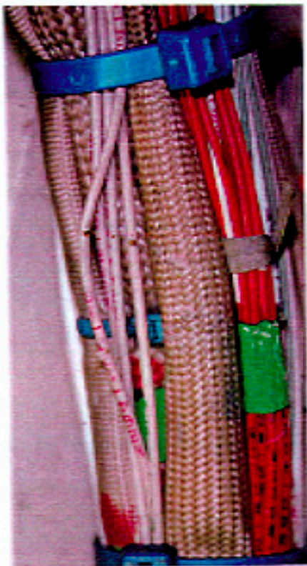
Wire damage at location A in Figure B-2. Three wires affected in addition to scuffing of braided sheath.
