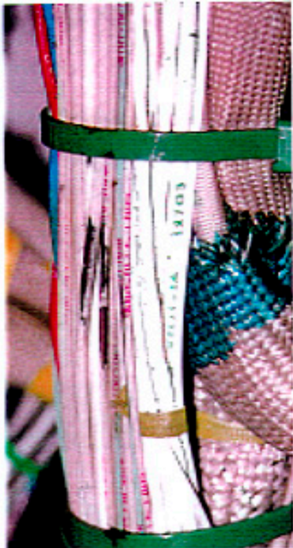
Abrasion of insulation topcoat at location B in Figure B-2.
