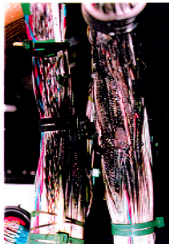
Detail view of failed areas of loom, and the adjacent heat affected loom. Above is a sketch of a cross section of the failed loom at the identified position.
