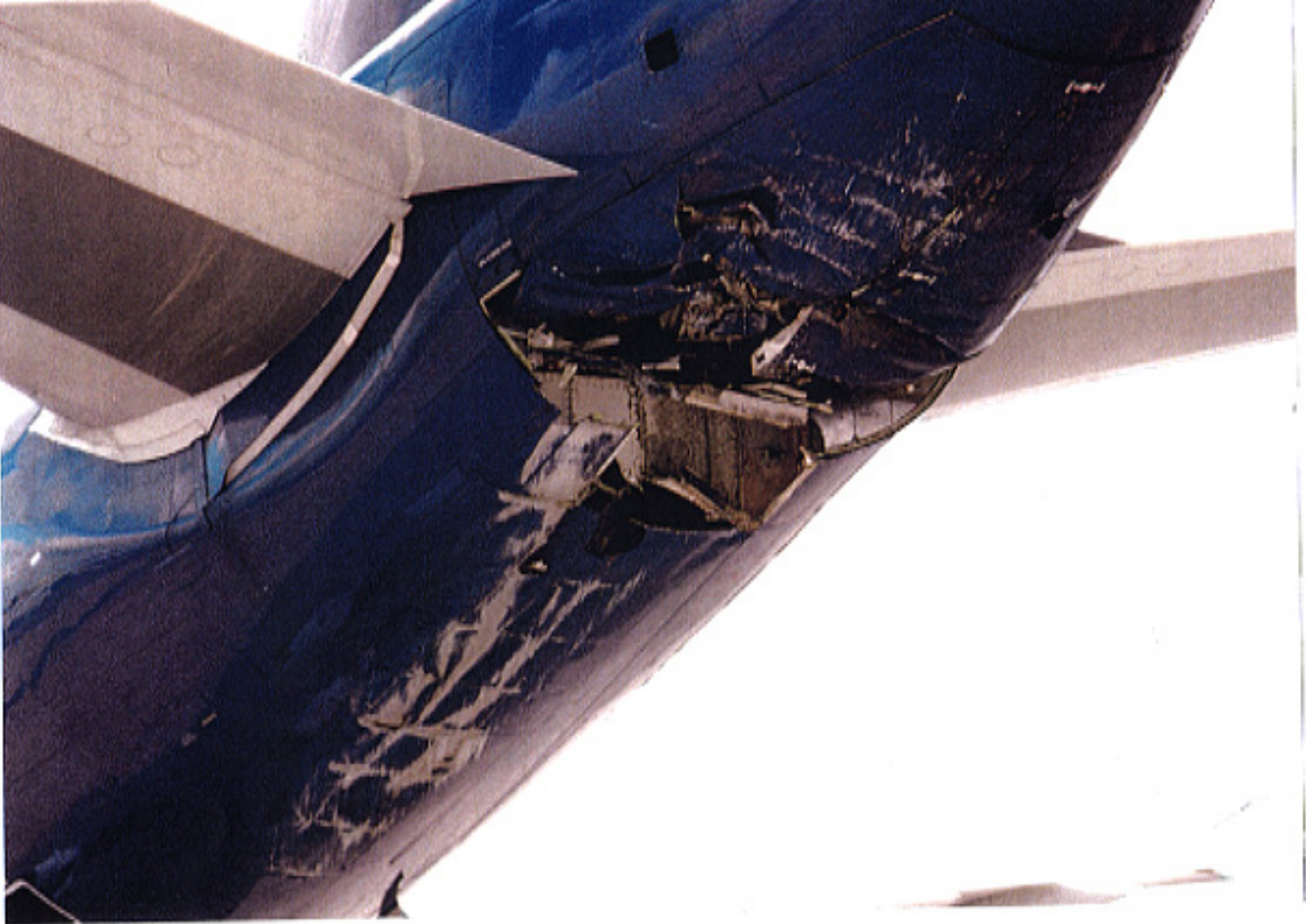
Figure 3 View of damage to rear fuselage
