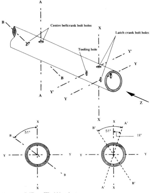
View on arrow Z. NB: axes XX and AA are shown coincident, although AA was in fact rotated appx  $1^{\circ}$  anticlockwise from XX
