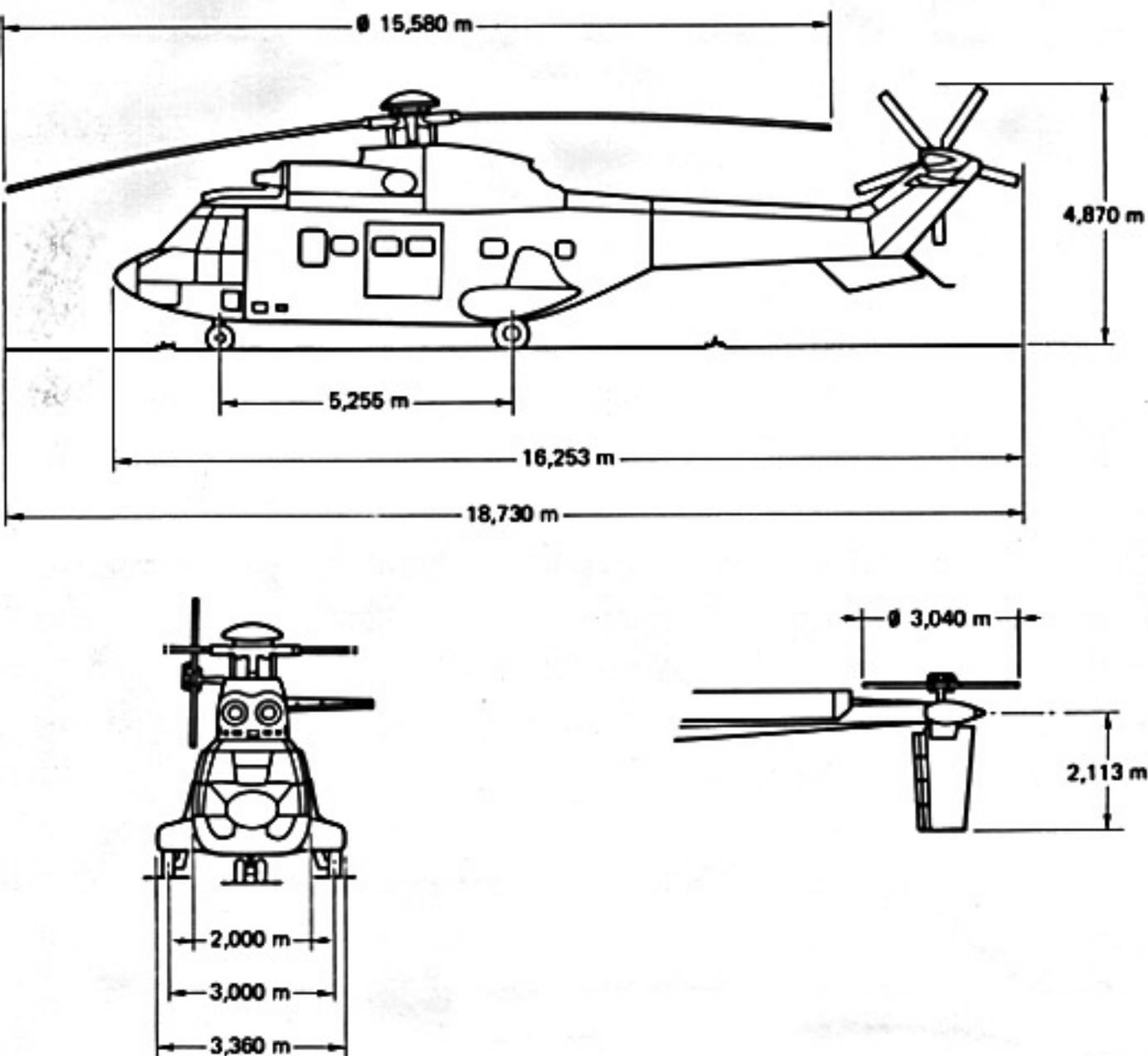
Figure 1: Showing general layout of AS332L
