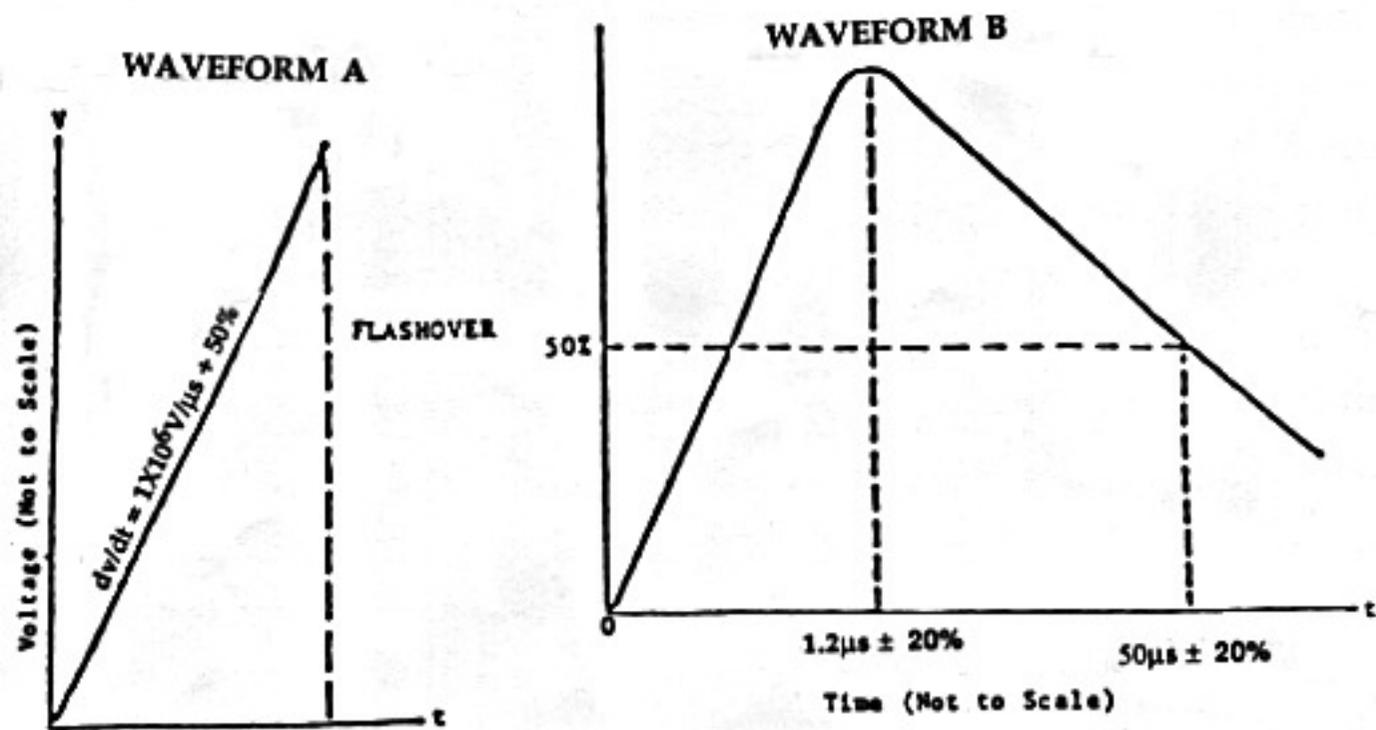
NOTE: Voltage Waveform "B" Full Wave - Waveform "B" rises to crest in 1.2  $\mu\text{s}$  (+20 percent). Time-to-crest and decay time (refer to open circuit voltage) of the lightning voltage generator, and assume that the waveform is not limited by puncture or flashover of the object under test.
