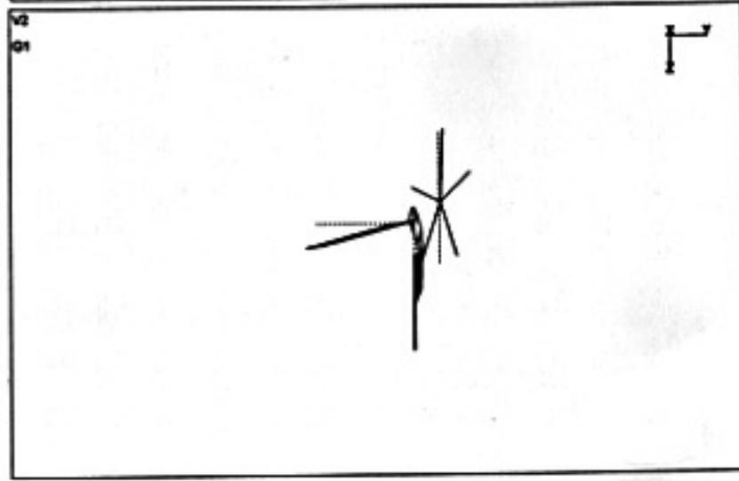
Figure 1: Showing predicted overtone vertical/lateral bending mode at 22.07Hz
