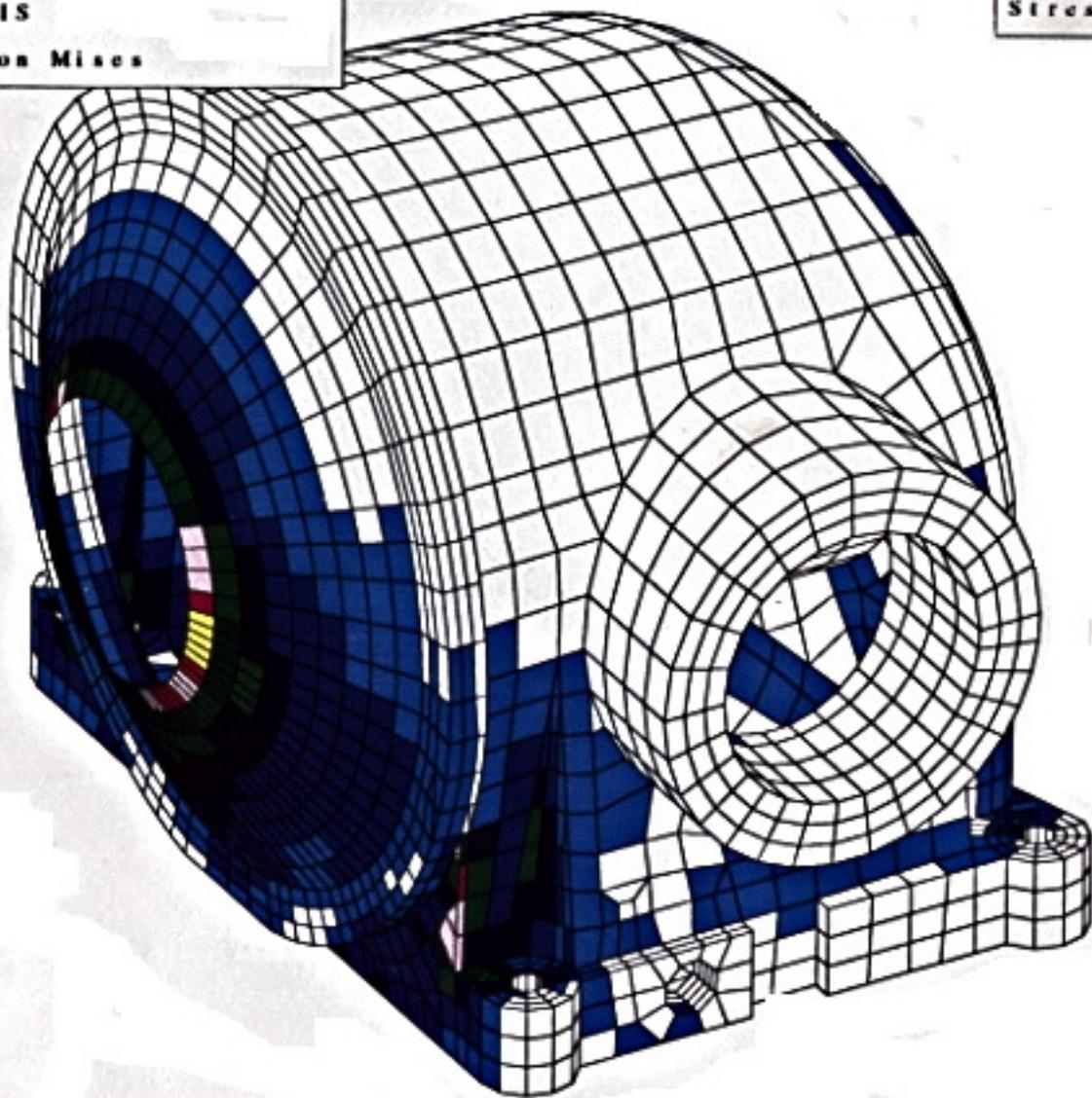
STRESSES DUE TO 100N LOADING IN Y-DIRECTION
