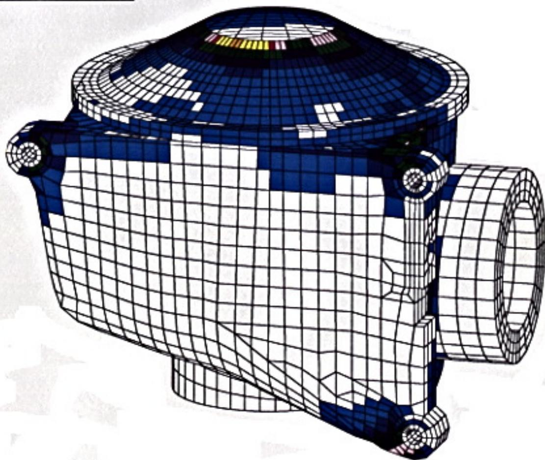
STRESSES DUE TO 100N LOADING IN X-DIRECTION
