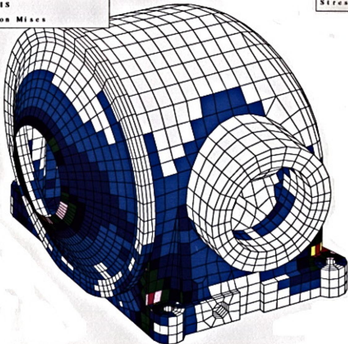
STRESSES DUE TO 100N LOADING IN X-DIRECTION
