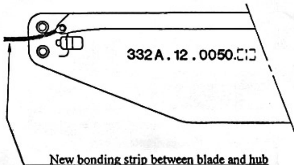
Figure 13C: Showing modified inboard conduction design with replacement of brass strip, which linked erosion shield to root bolt, by extended titanium shield, and fitment of single bonding strap.
