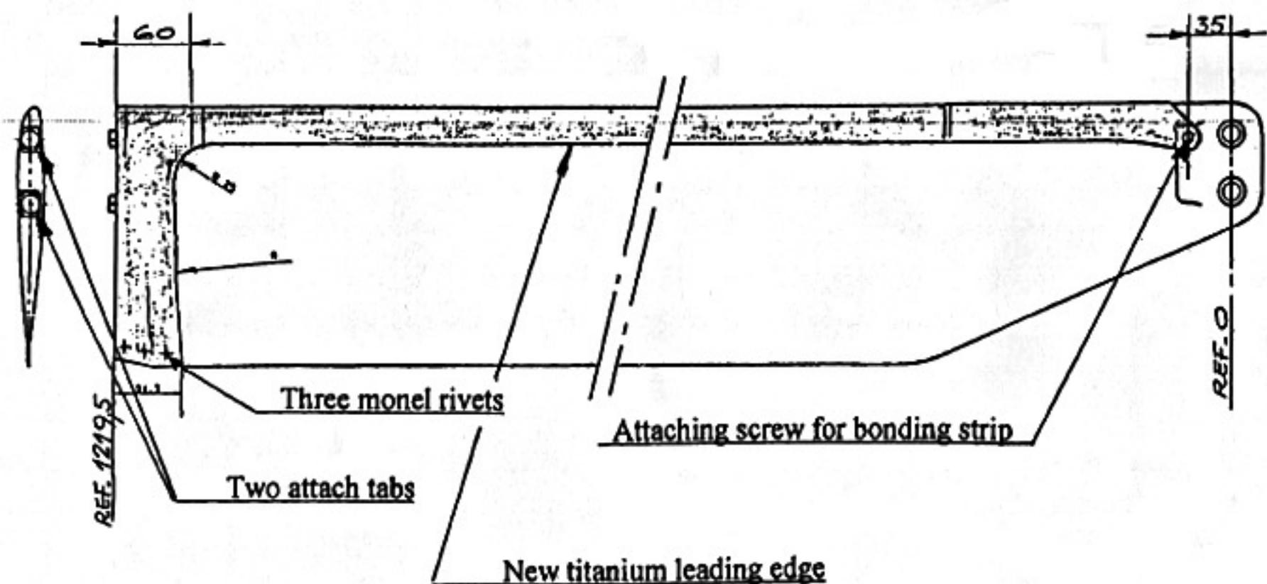
Figure 13B: Showing modified blade p/n 332A.12.0050 design with anti-erosion shield/conductor extended inboard to root and aft to provide improved blade tip conduction, with titanium 'tab' continuity to both tip weight bolts and rivetted attachment to trailing edge.
