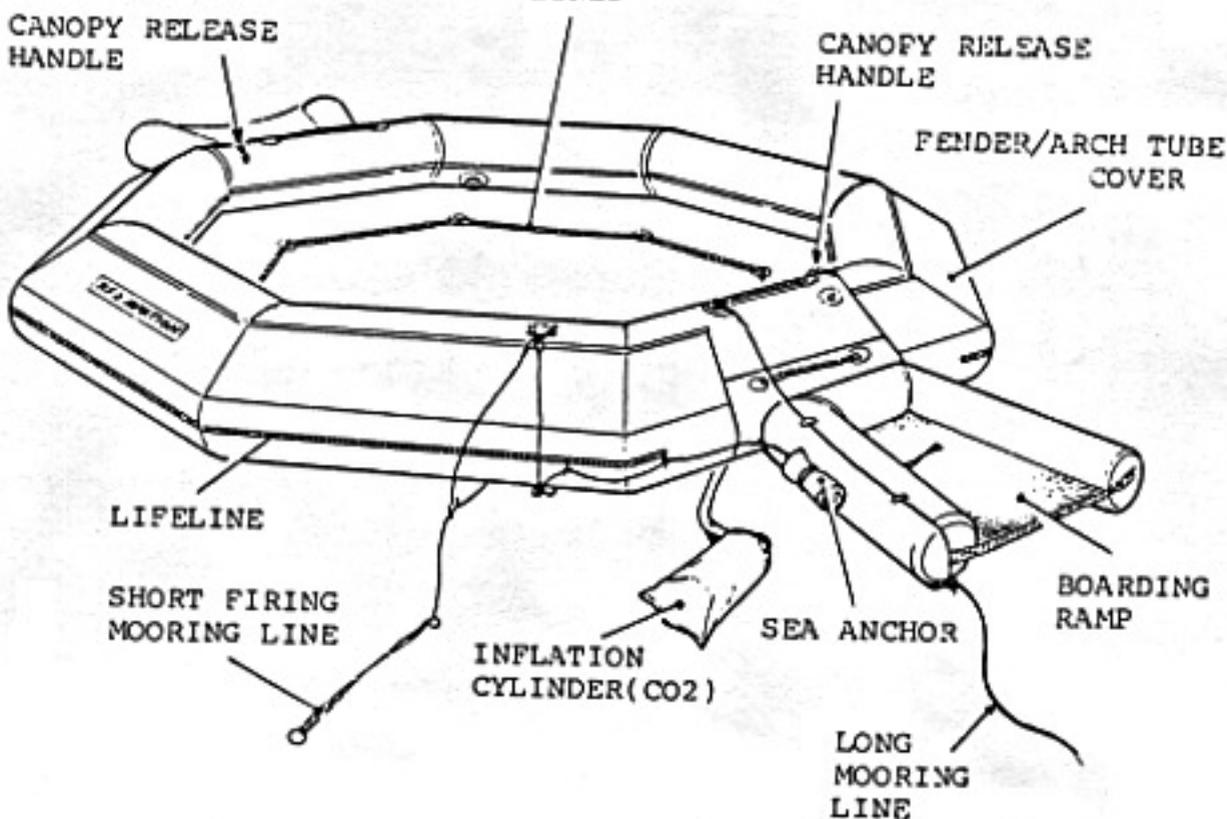
Figure 3: Showing general design features of the RFD Type 14R MK1 Liferaft.
