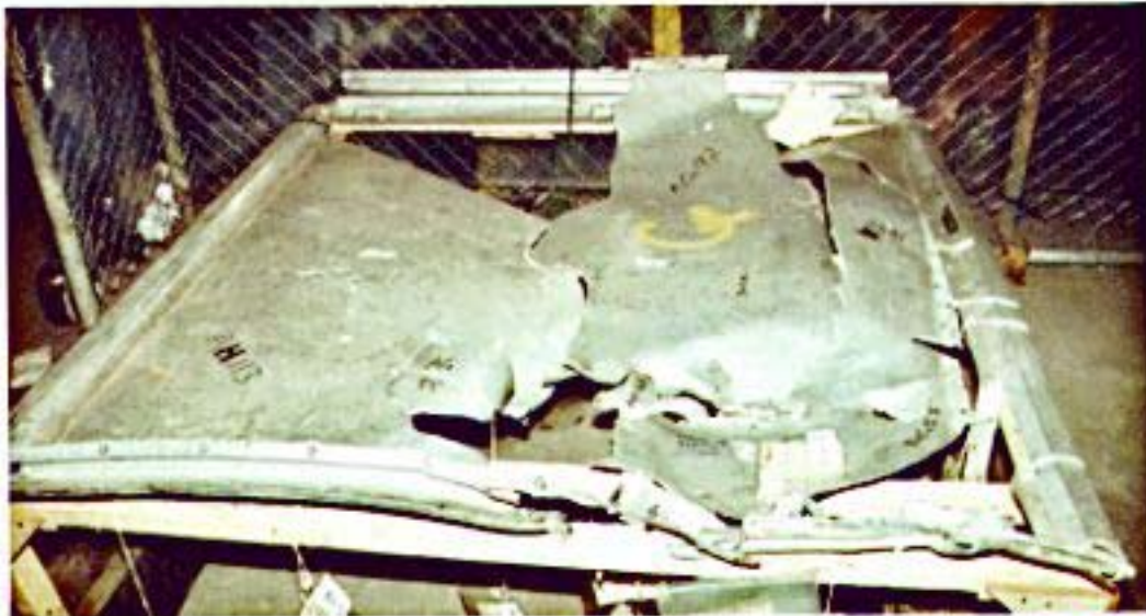
Detail of Damage to Container Floor
