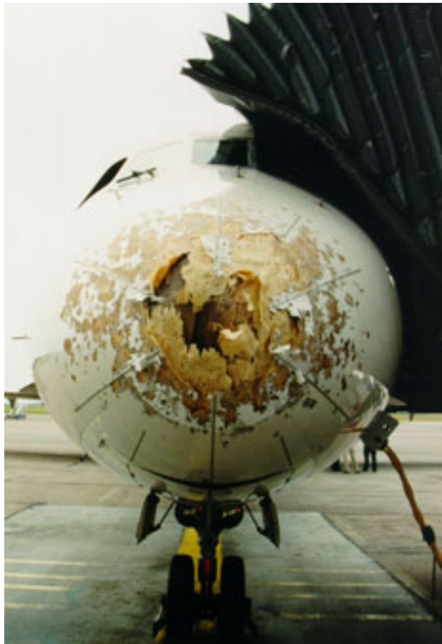
Figure 5. The damaged radome
