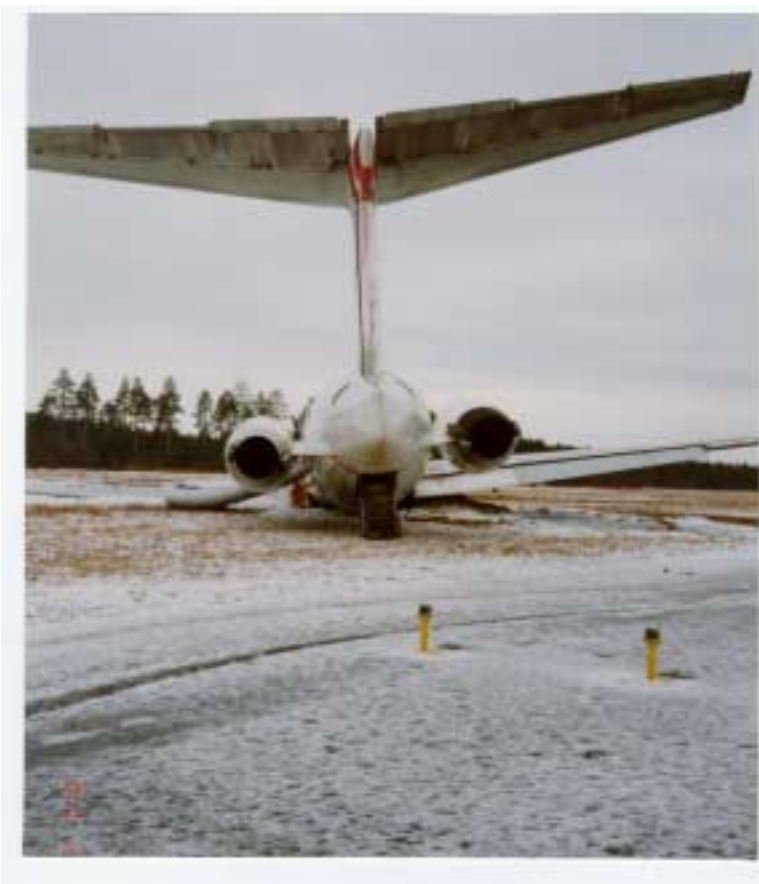
Figure 4. The evacuation of passengers through the aft stairs was not possible because the stairs did not have enough room to extend. The aft fuselage was lower than normal. The aft emergency exit would have been usable for evacuation.
