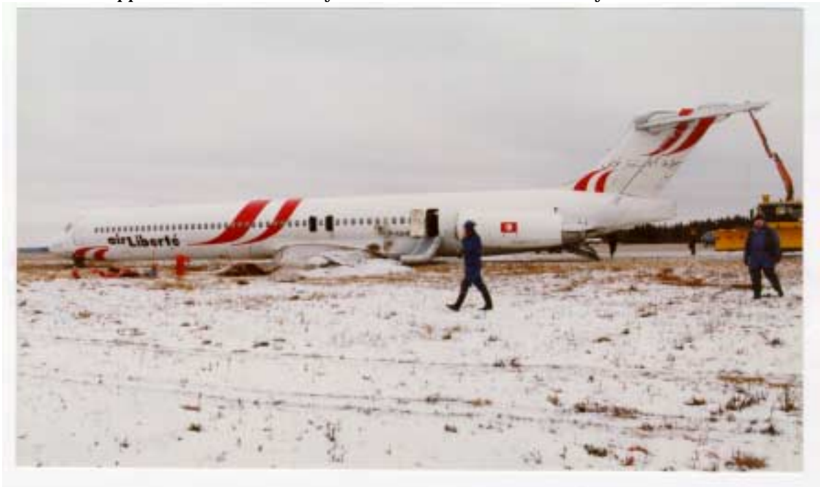
Figure 2. The left main landing gear has folded inboard into wheel well and the left wing has been damaged. Left wing fuel tank has got a leak. The evacuation took place through the aft galley service door and the left overwing emergency exits excluding two passengers who came out through the right overwing emergency exits.
