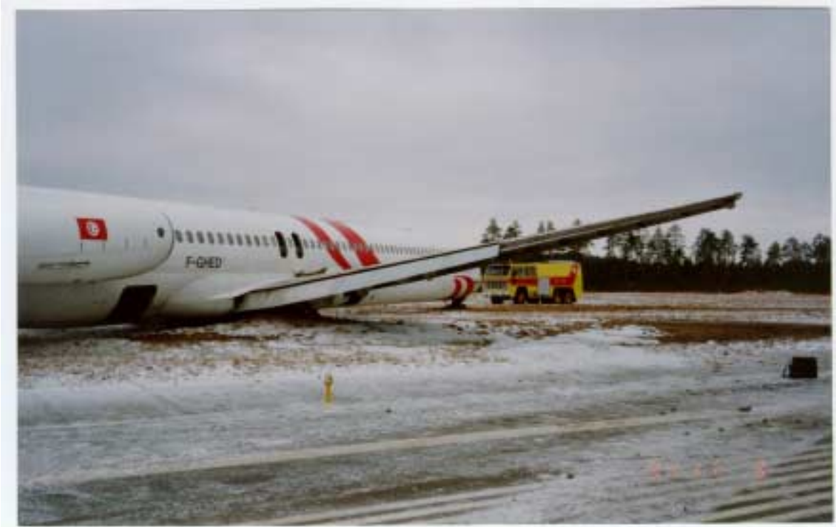
Figure 3. The right main landing gear has dug into the ground. The fuselage is lower than normal.
