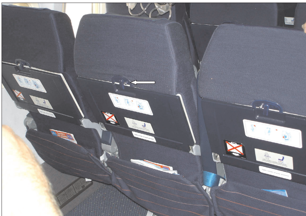
Figure 1.15.1.1. The latch of the meal table of the centre seat may rotate towards the sense of the Type III emergency exit escape path (to the left of the photo) and therefore it could be released during the emergency evacuation
