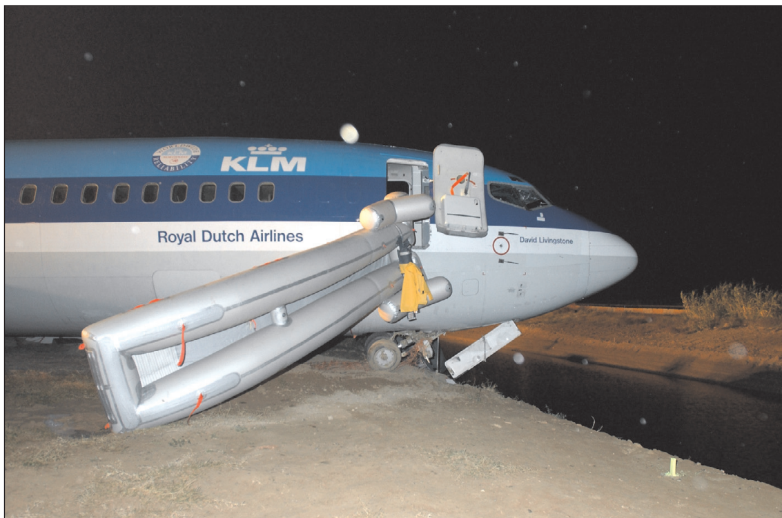
Figure 1.15.2. Escape slide of door 1R was twisted
