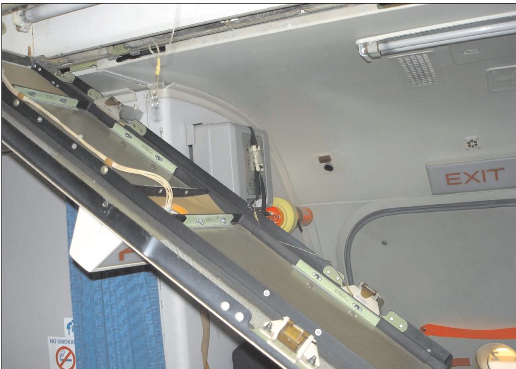
Figure 1.15.1.4. Ceiling panel in the rear cabin attendant compartment. During the inspection after the accident it was found closed, but witnesses stated that it opened after the aircraft came to a stop, therefore obstructing the path towards emergency exits L2 and R2. The lanyard released. The hook is at the end of the lanyard assembly
