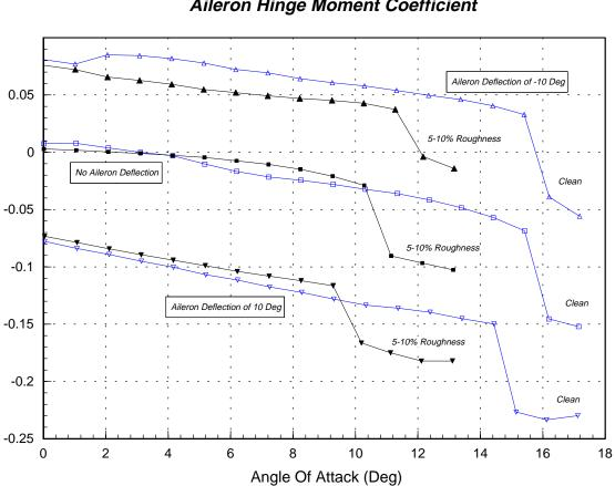
FAA/Univ of Illinois Wind Tunnel Data NACA 23012 Airfoil with Aileron Deflection Aileron Hinge Moment Coefficient APPENDIX H—COMAIR ICING GUIDANCE/PROCEDURES
