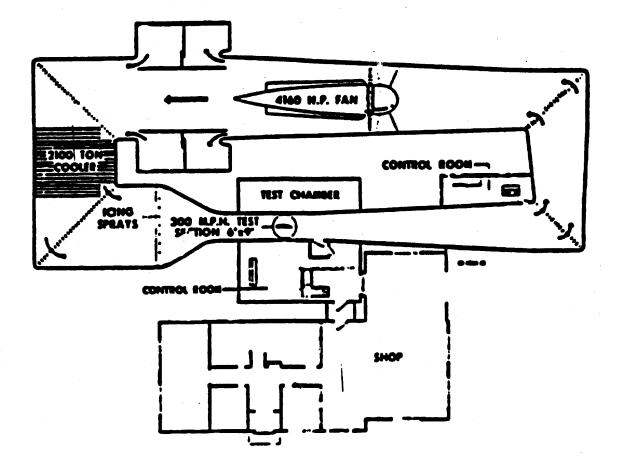
Figure 12.--NASA Lewis Icing Research Tunnel.
