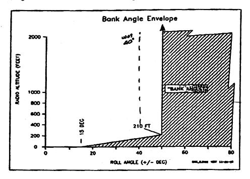
Figure 6.6.2-1: Excessive Bank Angle Alert Envelope
