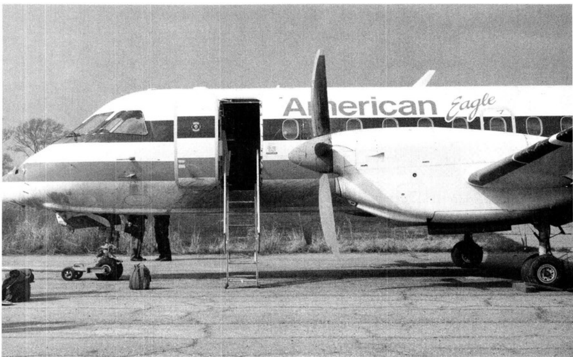
Figure 2b.--Airplane after recovery showing radome, puncture (in front of logo), and dented leading edge of wing.
