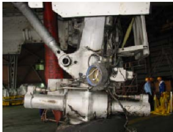
Figure 1.12-3NLG without broken sliding tube
