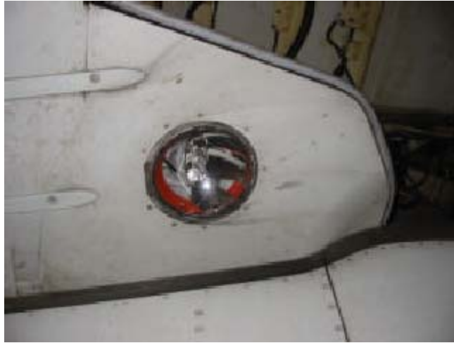
Figure 1.12-11 Landing light damaged
