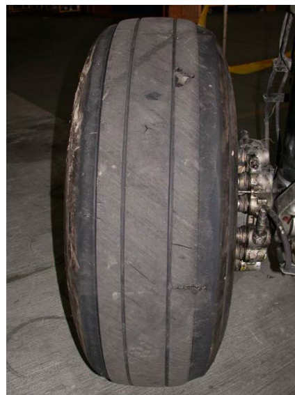
Figure 1.16-1 Deep cut damage and diagonal scratch marks
