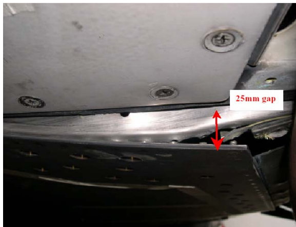
Figure 1.12-18 Internal profile deformed.
