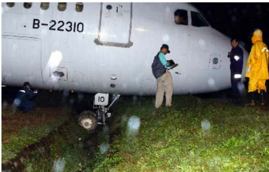
Figure 1.3-2 The NLG entered a drainage ditch (approx 1m deep)
