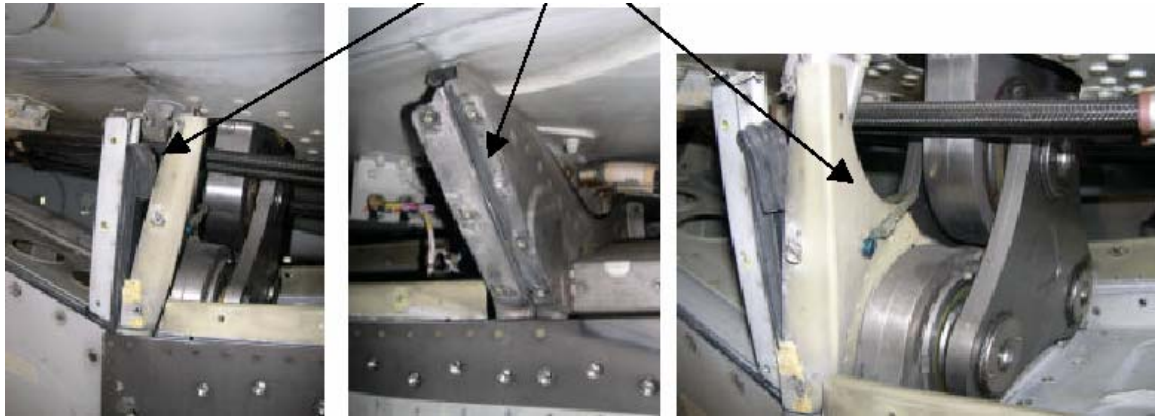
Figure 1.12-20 Vertical Profiles deformed
