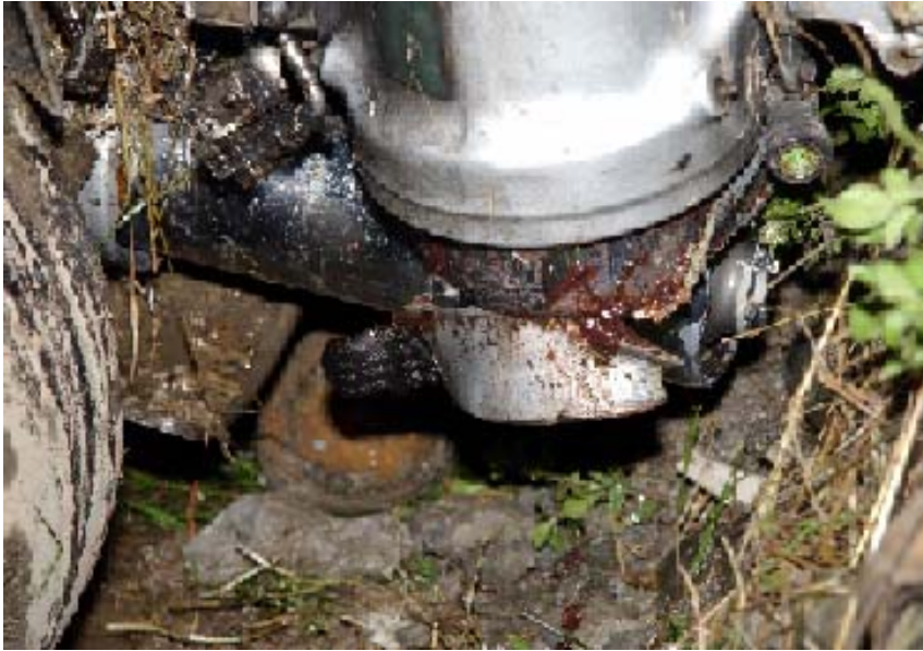
Figure 1.3-3 Sliding tube of the nose gear was broken
