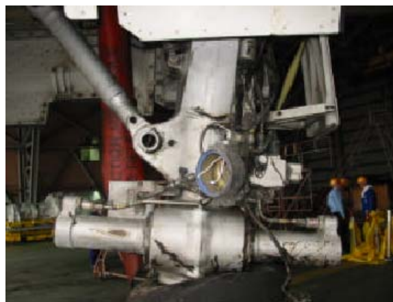
Figure 1.12-3NLG without broken sliding tube
