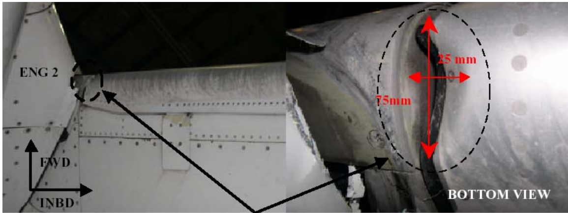
Figure 1.12-23 leading edge lower skin exhibited a 25mm x75mm dent
