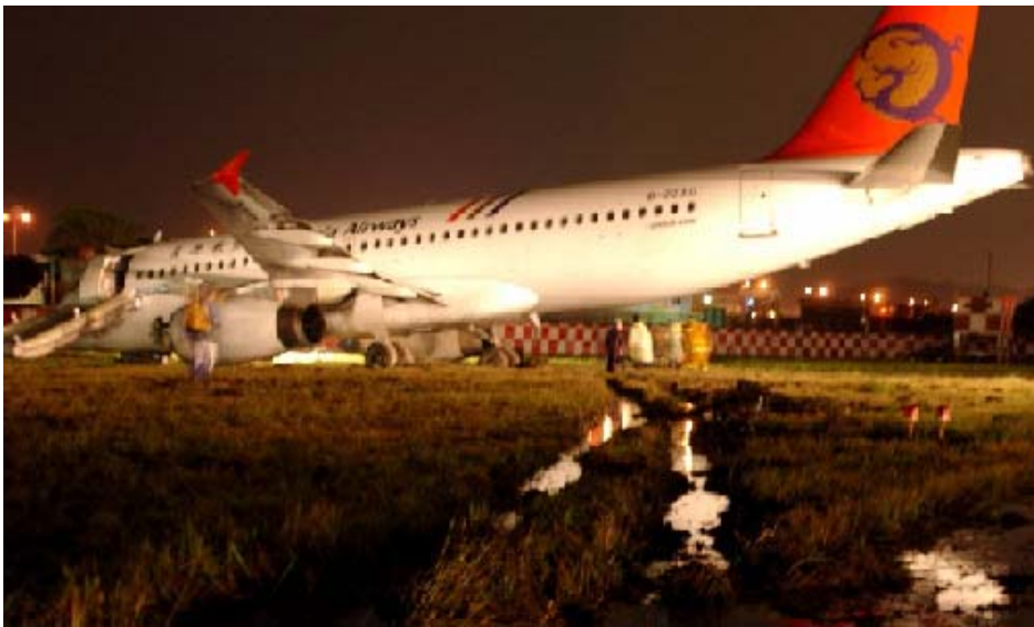
Figure 1.3-1 The aircraft rolled off runway and came to rest in a muddy area 90 degrees to the runway heading
