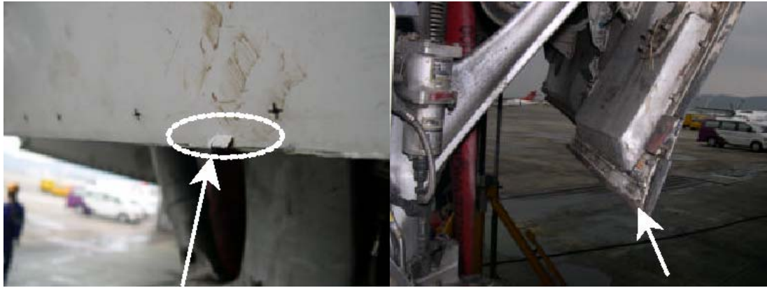
Figure 1.12-4 Deformation and dent to NLG Aft doors
