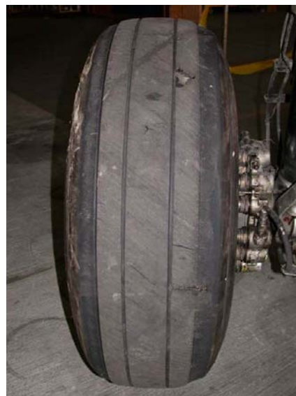
Figure 1.16-1 Deep cut damage and diagonal scratch marks
