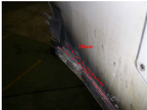
Figure 1.12-19 Twisting of the lower profile
