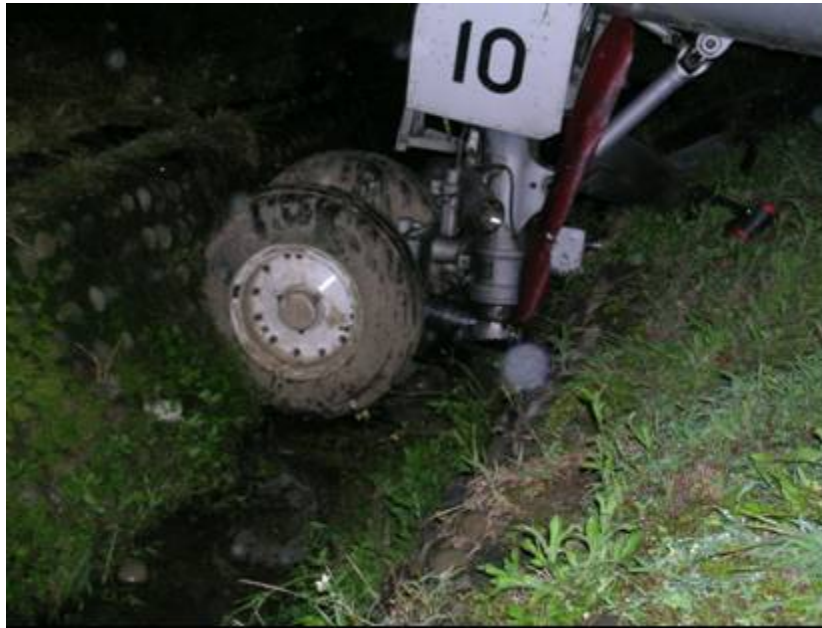
Figure 1.18-2 The nose gear stopped in the ditch
