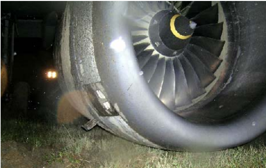
Figure 1.3-4 Both engine nacelles came in contact with the ground
