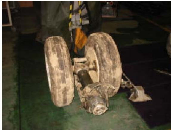
Figure 1.12-2NLG Sliding tube broken and associated harnesses destroyed
