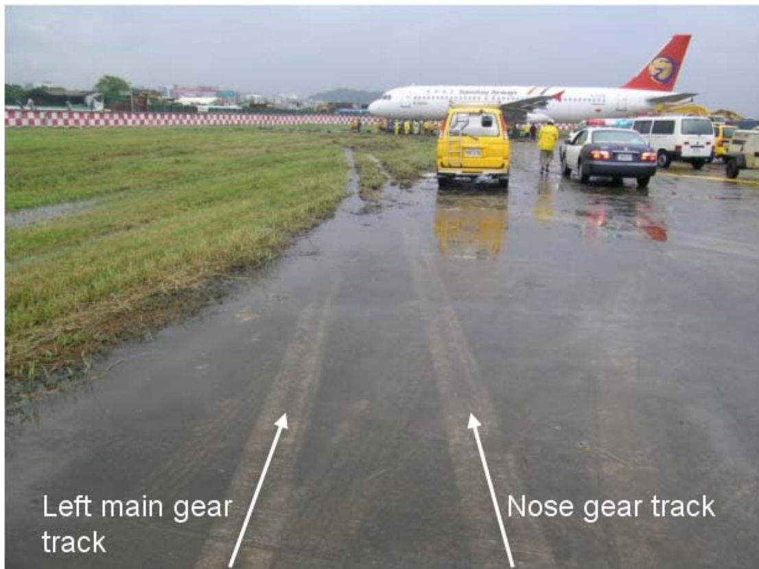
Figure 1.18-3 Ground tracks from the stopway pavement to the grass area
