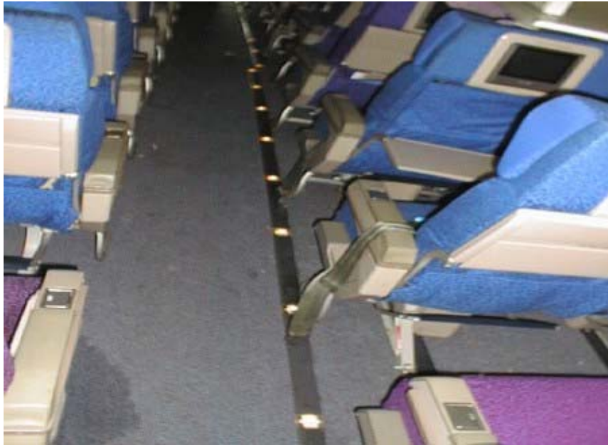
Figure 1.16-3 Illuminated floor proximity lights in aft fuselage section during testing
