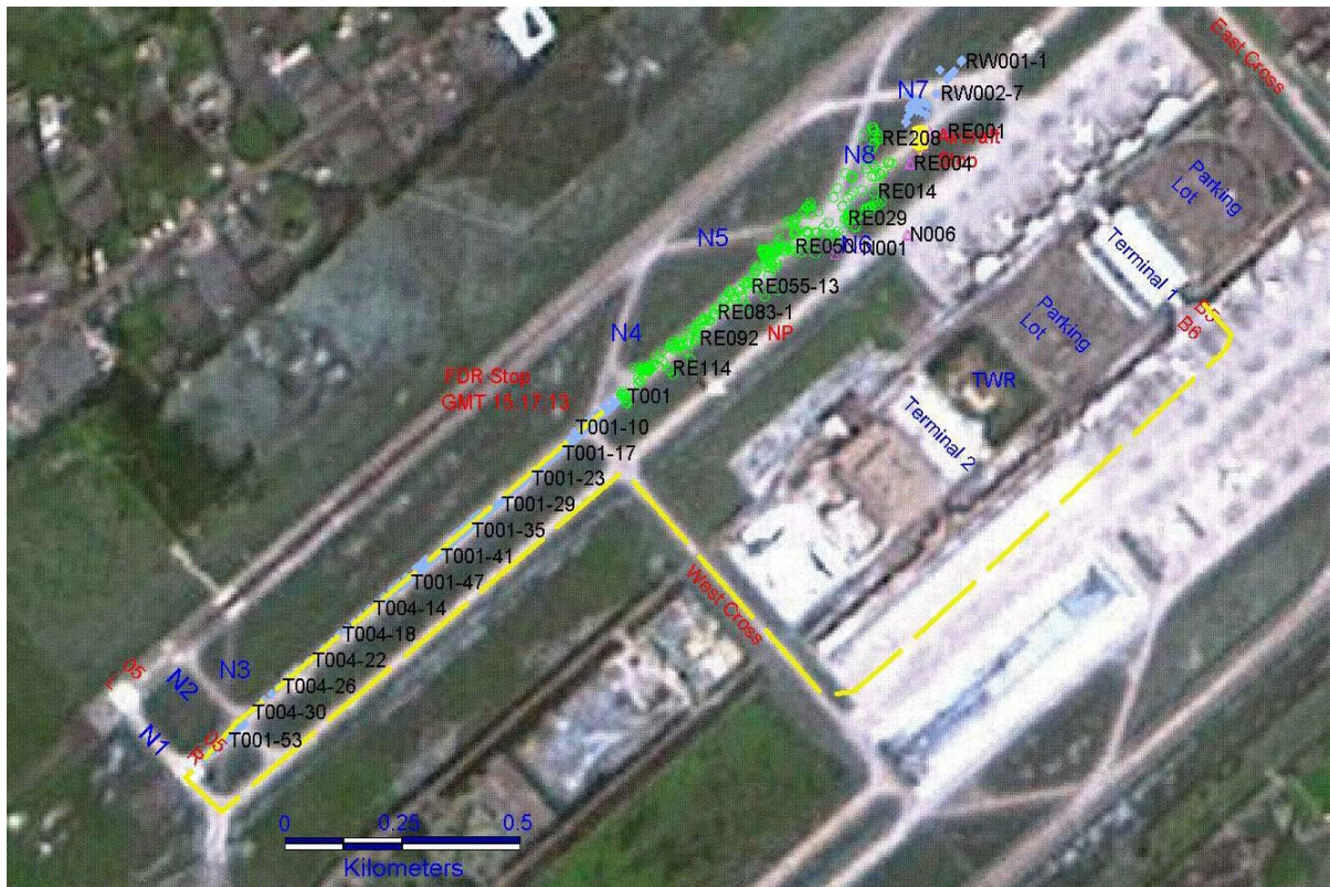
Figure 1.11-1 The combination of FDR data, site survey data, and the satellite map
