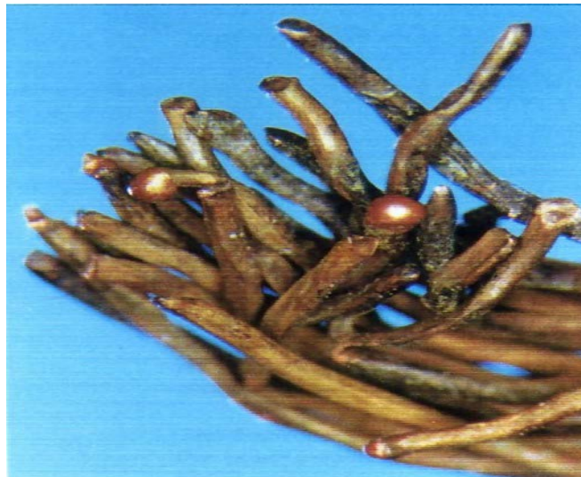
Figure 1.16-6 RE240-1, some of the melting beads formed at wire ends.
