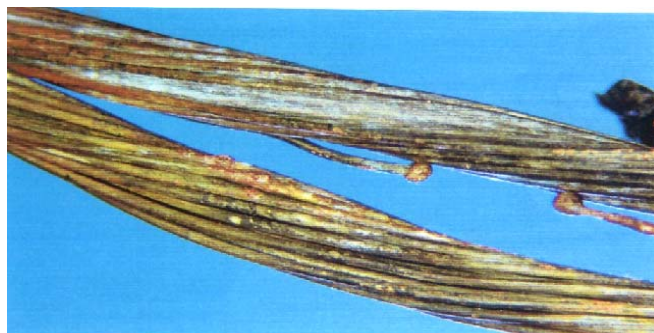
Figure 1.16-7 RE240-1, localized melting near the boundary of insulation that was lost.
