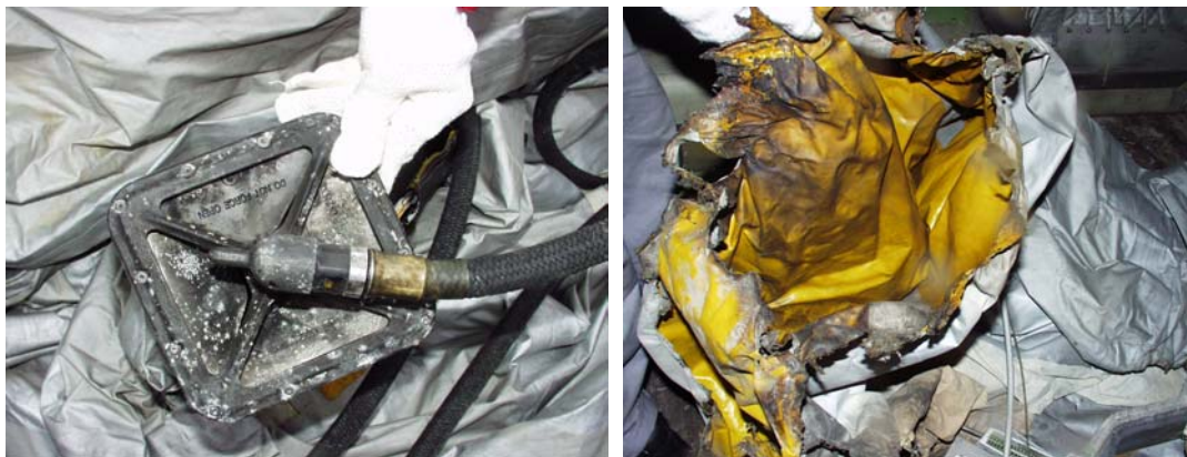
Figure 1.12-11 The aspirator inlet (left) and the inner fire damage of 4R slide (right)
