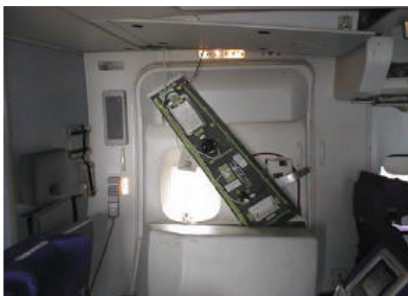
Figure 1.3-2 Illuminated Door 5 Left Emergency Light during testing (The over door fairing panel was removed to access the emergency light battery check)
