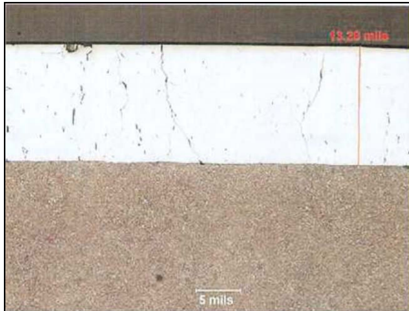
Cross section through the chrome plating showing the through-thickness cracks. (Courtesy of The Boeing Company)
