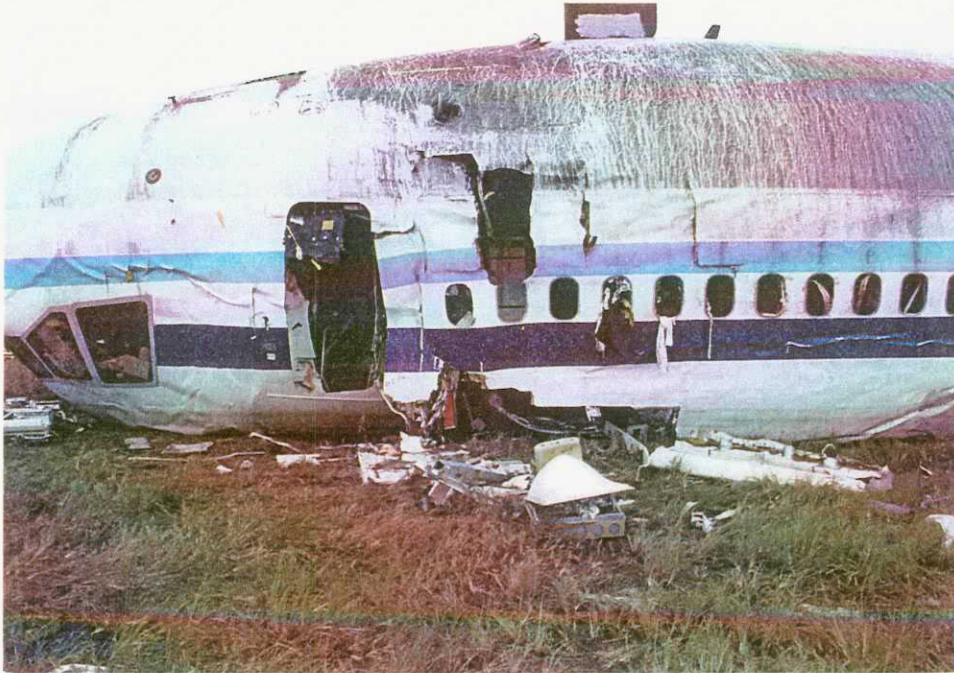
6. View of right side of fuselage including Door 1R.
