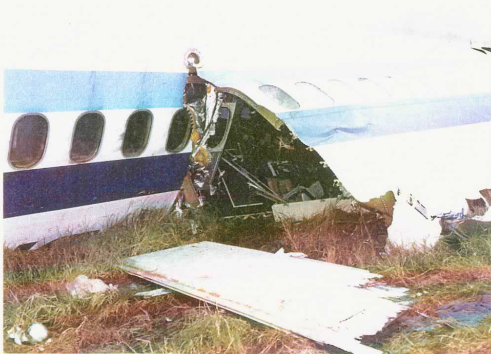
9. View of crack in right fuselage (aft).
