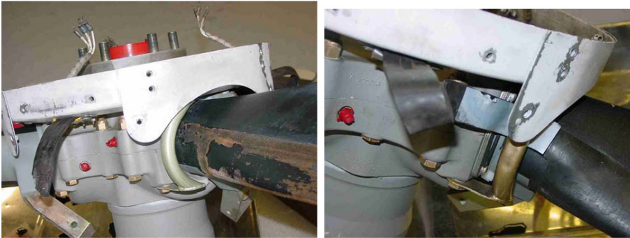
Figure 6: Second fracture in strap, near electrical termination
