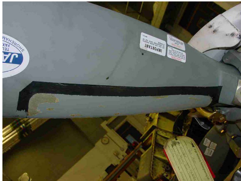
Figure 8: Aft surface of Blade 2 after removal of de-icer boot
