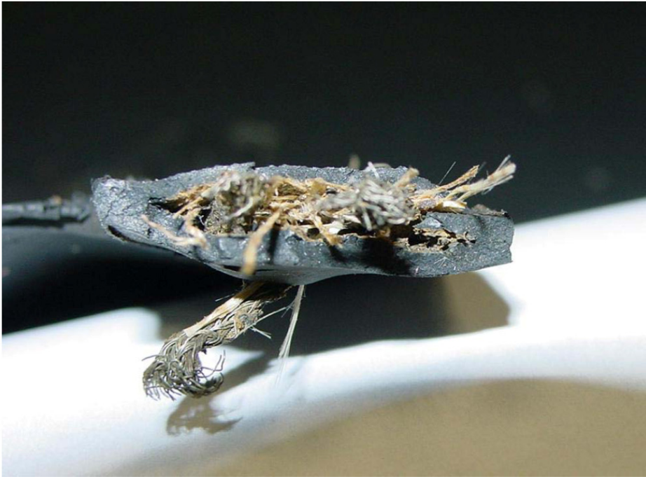
Figure 4: Rubber failure at the root end of boot from Blade 1
