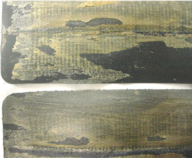
Figure 12: Comparison of colouration of de-icer boots removed from Blades 3 (top) and 2 (bottom), showing discolouration of the former with time
