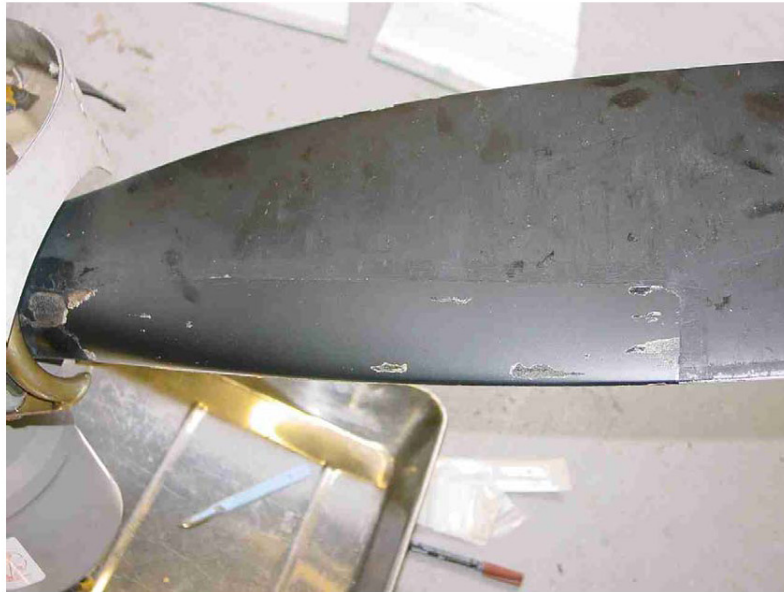
Figure 8: Aft surface of Blade 2 after removal of de-icer boot
