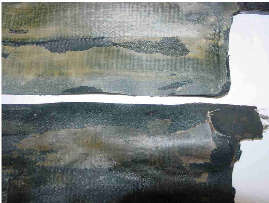
Figure 11: Comparison of adhesive colouration on de-icer boots from Blades 1 (bottom) and 2 (top)
