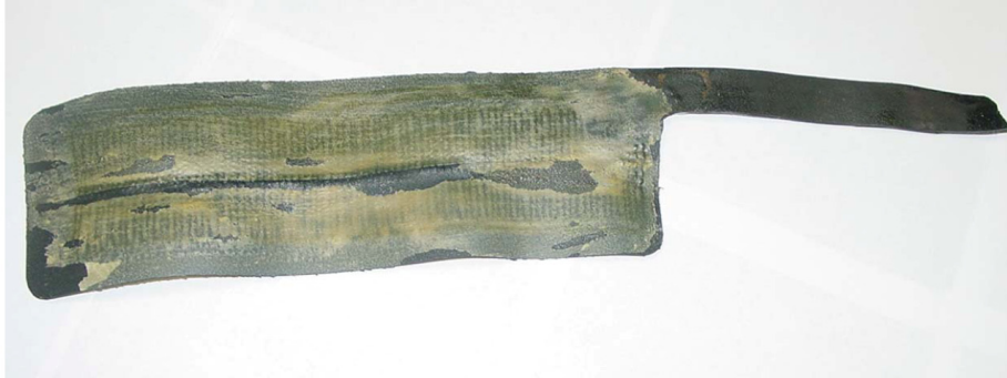
Figure 10: De-icer boot removed from Blade 2
