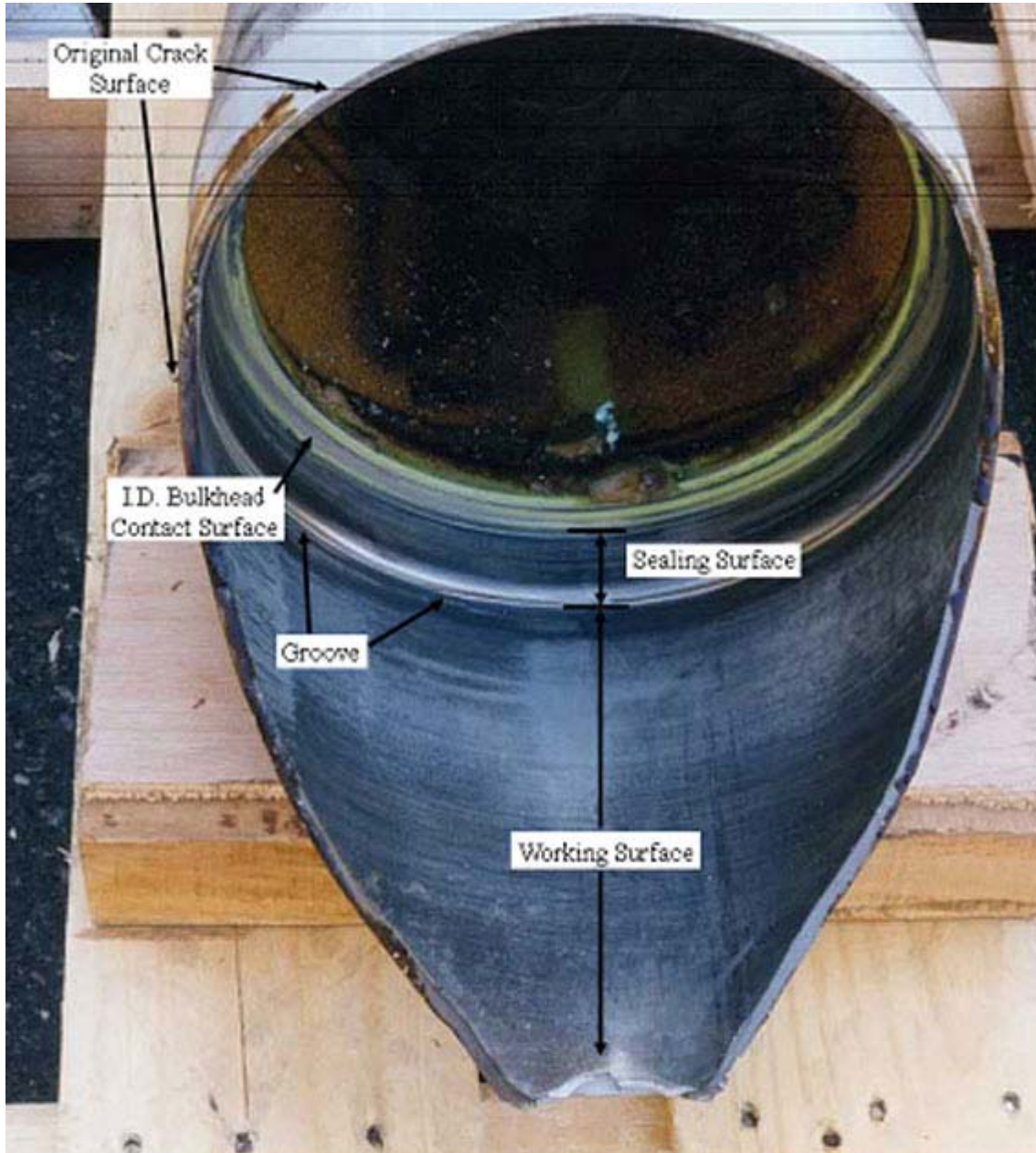
Nose landing gear outer cylinder that was involved in the 1998 incident showing the area of failure (Photograph courtesy of Boeing Materials Technology)
