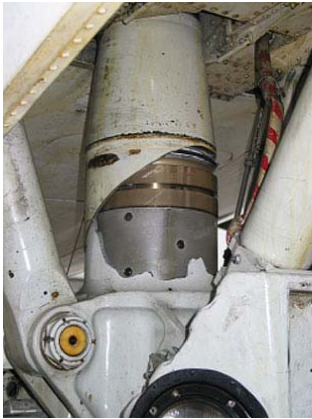
Nose landing gear outer cylinder showing the area from which the ejected section of cylinder material originated
