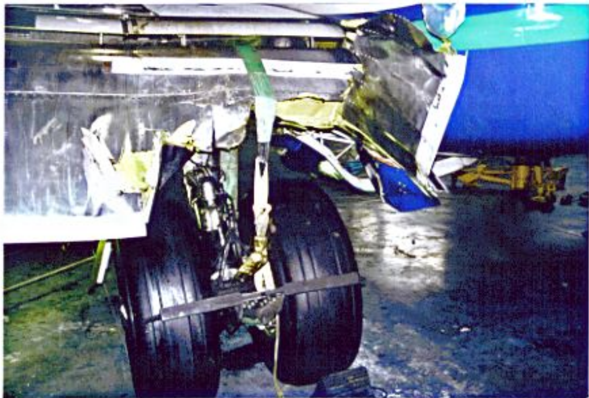
G-DEVR on jacks post-accident. View of left MLG from aft looking forward showing damage to trailing edge flaps
