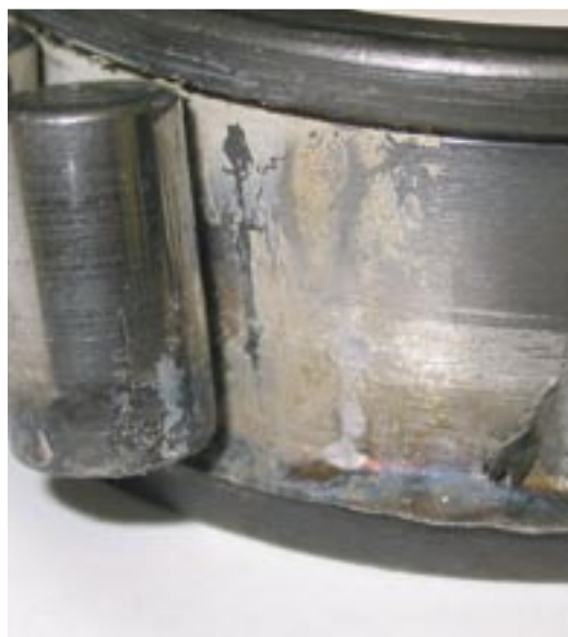
Figure 7 (right) Distortion of cone large rib face
