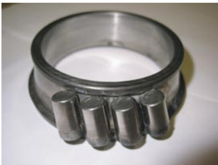
Figure 6 (left) Rollers welded to cone
